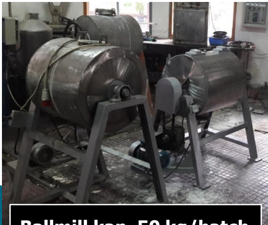
Ballmill kap. 50 kg/batch
